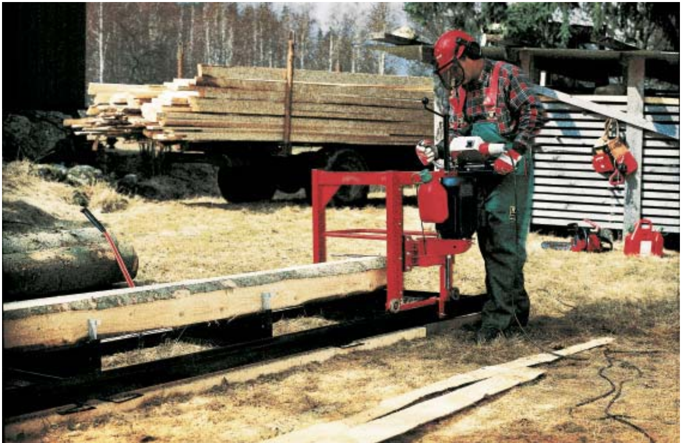
Fig. 11. The Lennartfors SM2186 Chain Saw Mill.
